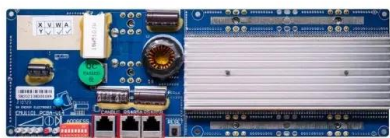
ESM5 * Communication between battery and server Band rate: 9600bps ESM5 Interface * Communication between stacked packs or EMS and PC Band rate: 9600bps
