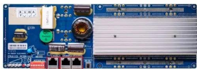
RS485 Communication between battery and inverters Board size: 9000mm RS485 Interface Communication between parallel packs or BMS and PC Board size: 9000mm
